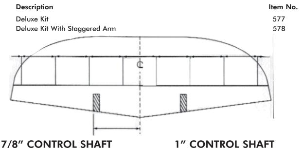
Drilled and spotfaced to receive our 3/4" stainless control arms. This control shaft is furnished with our deluxe adjustable plate kit. Accompany order with layout on above diagram to facilitate drilling and spotfacing.
